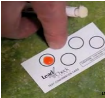
If the surface tests negative, verify the validity of the test with the calibration card provided.
