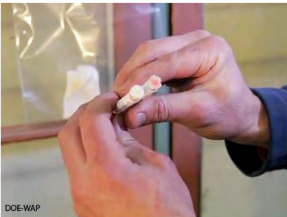
First, crush the capsule and shake it to mix ingredients. Then swab the sample for 30 seconds.
